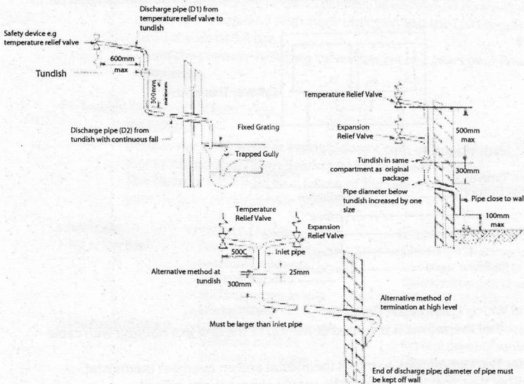
Note: The discharge will consist of scalding water and steam. Asphalt, roofing felt and nonmetallic rainwater goods may be damaged by such discharges.
